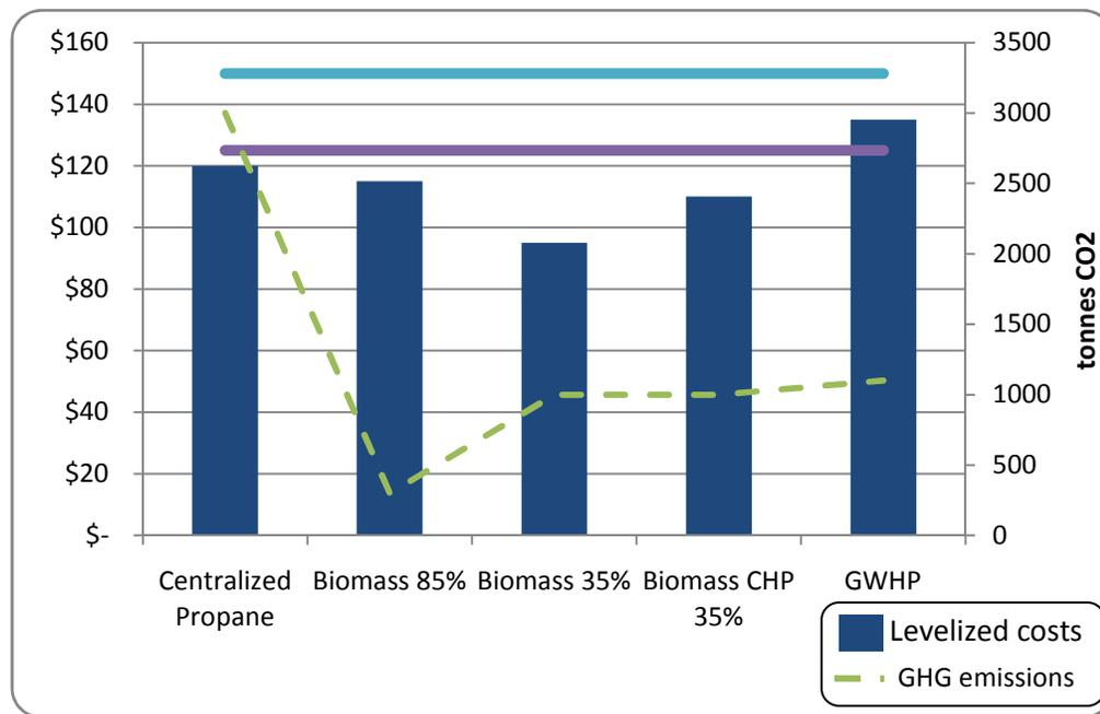
Biomass sized to 35% of peak heating demand has the lowest levelized cost. For biomass CHP sized to 35% of peak demand to be competitive with heating-only biomass sized to 35% of peak demand, the electricity purchase price would have to be over \$300 per MW.h. All of these costs are based on free biomass fuel.
