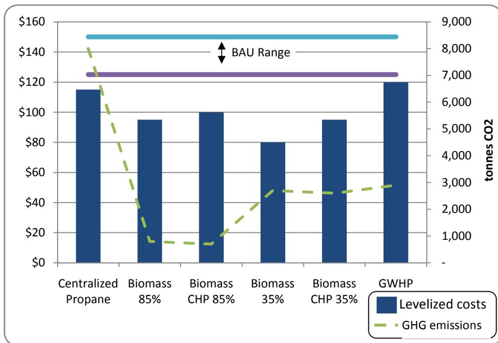
For a viable district heating system, DPS costs would typically be 5 – 12% of total levelized costs. Given the BAU range of \$125 – \$150 per MW.h, this would be equivalent to \$6 – \$18 per MW.h. As the lowest-cost option, heating-only biomass sized to 35% of peak demand, has an available residual of \$45 compared to the low end of the BAU range, it appears as though there is sufficient residual to cover DPS costs, with excess funds available for phasing costs and other system costs.
